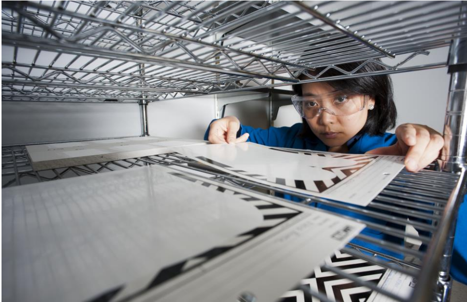
Product test: an employee checks panels coated with VAE-based interior architectural paints drying on a rack. The VAE dispersion VINNAPAS® EP 3360 ULS enables the formulation of high-performance interior paints with reduced emissions (photo: Wacker Chemie AG).
