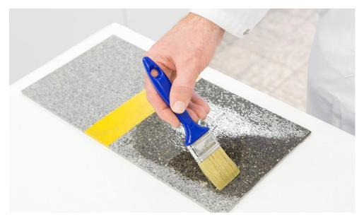
WACKER is presenting an innovative binder for the impregnation of cement-bound substrates. Tests have shown that SILRES<sup>®</sup> BS 6920 offers substrates effective protection against even stubborn stains. Even after several hours, red wine, coffee and oil can be wiped off without leaving any stains (photo: Wacker Chemie AG).
