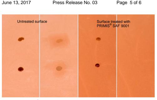
The new PRIMIS<sup>®</sup> SAF 9001 dispersion renders surfaces soiling resistant: on untreated decorative mineral floors, coffee and blackcurrant juice leave distinctive stains even after wiping with a wet sponge (left). On the treated flooring (right), both substances can easily be completely removed by moist wiping (photo: Wacker Chemie AG)
