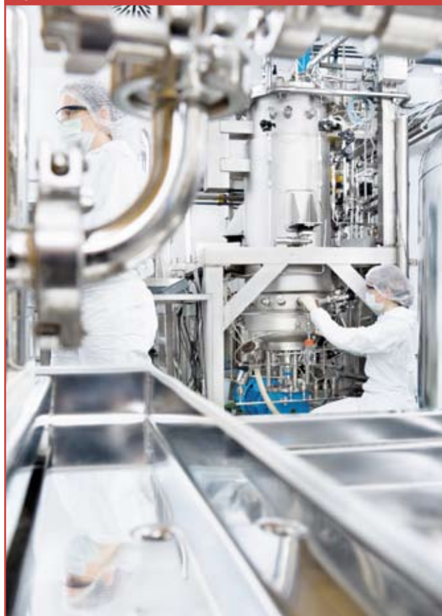
Figure 3: Production facility with 300 l fermenter at Wacker Biotech.
