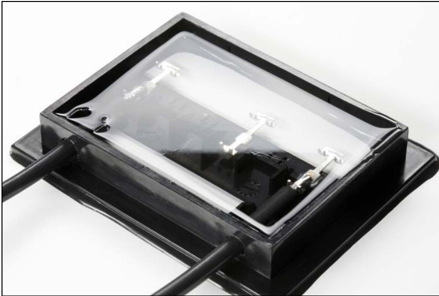
Junction box (without connections and bypass diodes) for a photovoltaic module, encapsulated in ELASTOSIL® Solar 2120 UV. The silicone is characterized by fast curing times at room temperature. Curing is initiated by UV light and not, as with conventional silicone elastomers, by heat. (Photo: Wacker Chemie AG)
