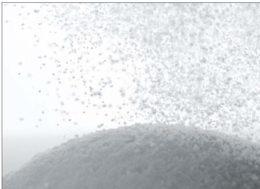
HDK ® pyrogenic silica from WACKER. Among the many applications of this high-purity powder are rheology control, reinforcement of silicone elastomers, silicon wafer polishing and thermal insulation materials (Photo: Wacker Chemie AG)
