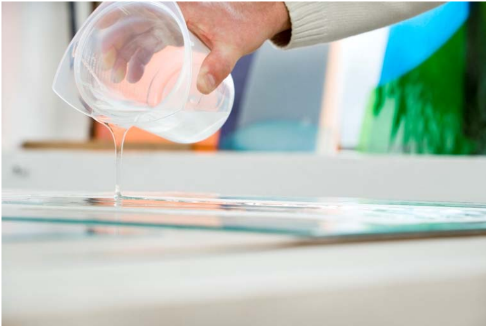
Bonding glass with WACKER SilGel® 612. The transparent, plasticizer-free silicone gel is pourable and therefore particularly easy to process. (photo: Wacker Chemie AG)
