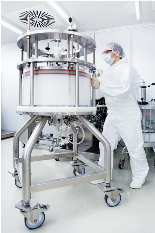
Cleanroom at the expanded Wacker Biotech facility in Jena: this is where biologics are produced. Downstream, the desired active protein is purified via chromatography (photo: Wacker Chemie AG).
