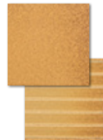
Example: Glazed ceramic tile, with a porous profile back pattern 6.0 < E_b \leq 10.0\%
