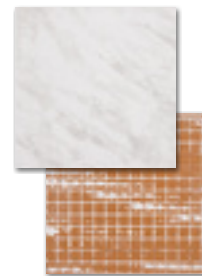
Example: Unglazed ceramic tile. This tile additionally has a 0.5 < E_b \leq 3.0\%
