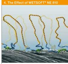
Hydrophilic polyglycol chains (blue) are attached via anchoring groups (green) directly to the fiber surface > hydrophilicity and softness
