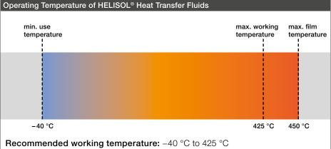
**Suggested applications:** CSP (concentrated solar power), process heat, heating/cooling applications
