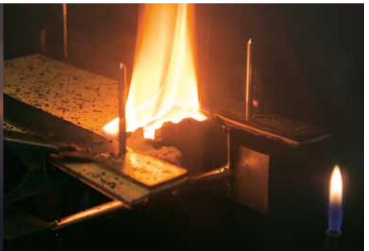
SB latex/calcium carbonate film (150% filler loading) according to DIN 4102-1.
