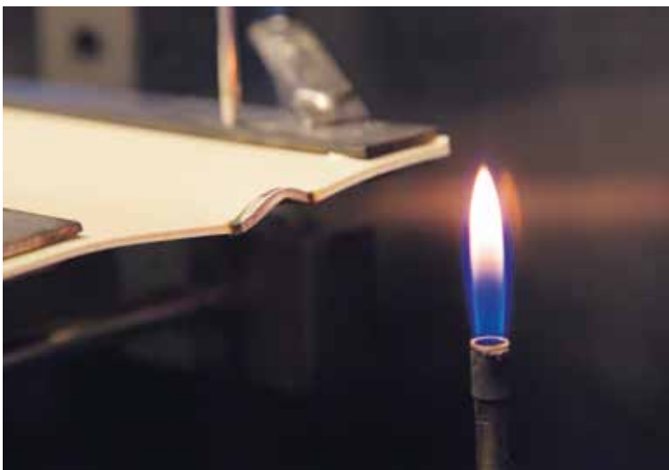
VAE/calcium carbonate film (150% filler loading according to DIN 4102-1; self-extinguishing.
