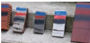
Left: different substrates treated with SILRES® BS 710, sprayed with typical graffiti paint (upper row) and then cleaned with water (lower row). Right: Graffiti can be removed just with pressurized water.
