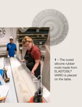
aligned. Round rosettes, for example, are made by hand by rotating them around their axes. This process creates the original shape from which the silicone rubber mold is made. "The traction phase requires the utmost precision. The reel must run smoothly, which is difficult if the molding is decorative. It doesn't want to be pulled," Hakala explains.
