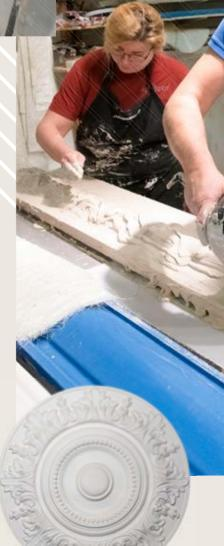
5 – After 21 minutes, the plaster is hardened and can be demolded from the silicone rubber mold.
