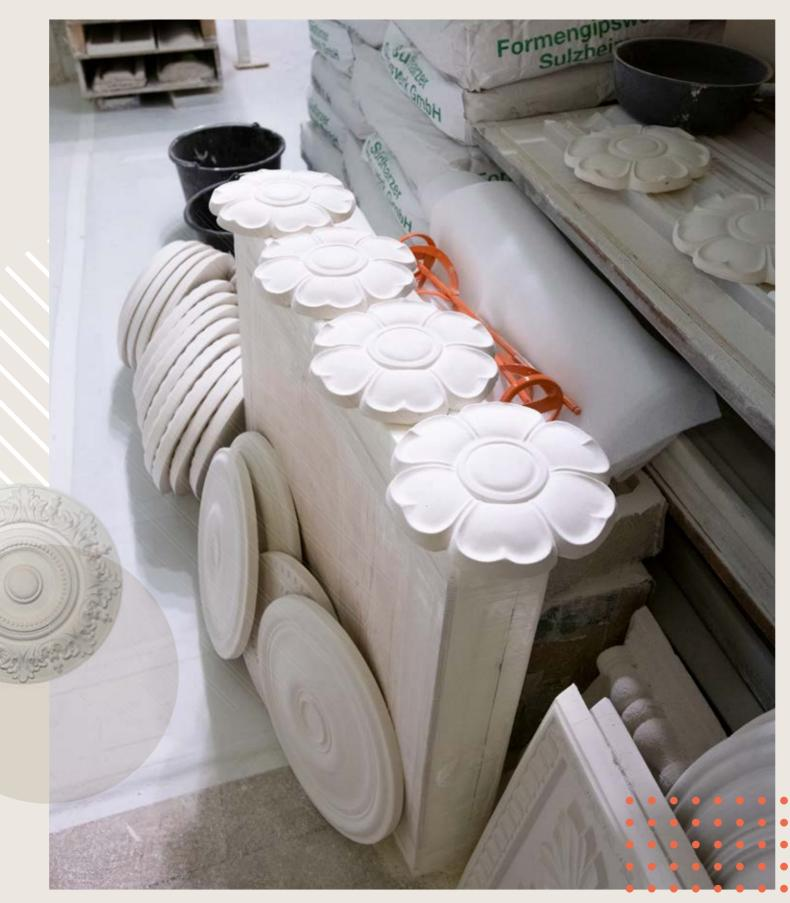
When the ceiling rosettes are released from the silicone mold, they replicate the historical original in every detail.
