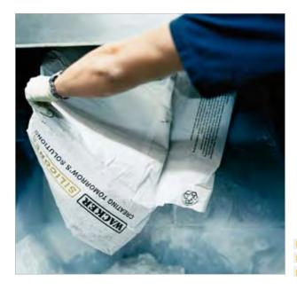
Pyrogenic silica from WACKER is processed by Sika into polyurethane adhesives.
