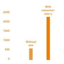
Joint fillers formulated with the new VINNAPAS® 4800 G gypsum binder offer greatly improved adhesion even to paper strips. The strips are often used to prevent cracks during the installation of plasterboard.
